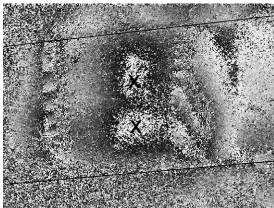
Figure 8. Fringe patterns recorded for a sample with I_c = 2 A under a 10 A current, at t = 35 s, showing two defects (marked with black crosses) separated 3 mm.
